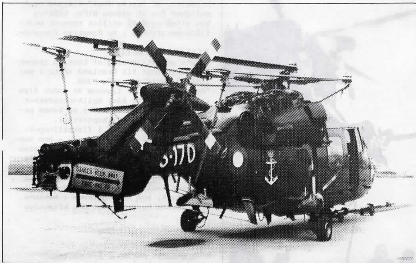
S-170 under foldningsøvelser på FSNVÆR 1980. En passende karakteristik kunne lyde: Rotary machinery, nautical style, a complicated collection of metal mechanisms and rotary reactions. - It works, too!
